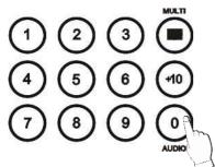
Audio ON/OFF: Press the FUNCTION button and then press the "AUDIO (0)" button to open/close the DVR audio function. You can hear audio of selected channel regardless of monitoring screen.
