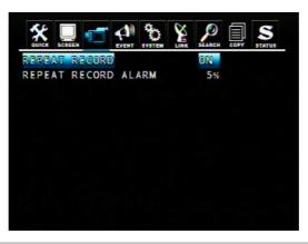
ON: When repeat recording, if the HDD is full, DVR will overwrite the recorded data automatically. OFF: Stop to record when the HDD is full.
