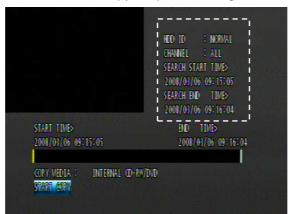
HDD ID: The HDD (HDD0, HDD1) which the record data saved. The default is NORMAL. The START TIME and END TIME of the selected record data will be shown on the screen.  $\circ$
