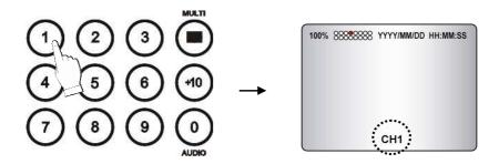
Press the desired camera number button to display on the monitor.
