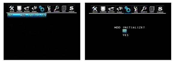
REC HDD INITIALIZE: Select YES and press ENTER button to format the HDD.
