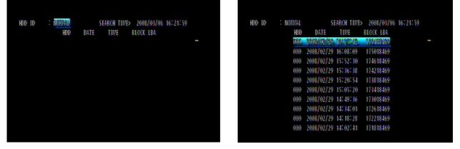
Select the desired HDD ID, TIME, BLOCK and press the ENTER button, the search relausts will be shown. Select the desired block and press ENTER to playback.
