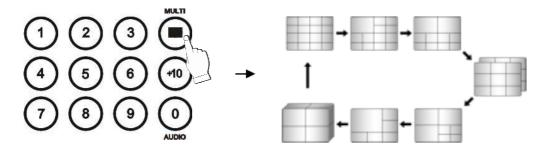
To change a single camera display to the multi camera, press the MULTI button.
