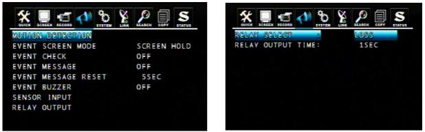
DVR provides a relay output interface; the following events will trigger off the relay signal:
