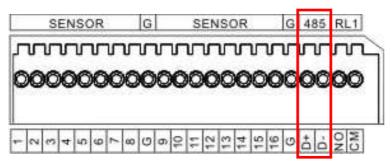
RS485 is use for connect to external device, such as keyboard or PTZ camera.
