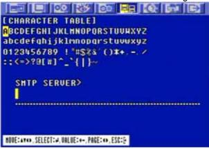
Select the character using the ♠ , ♣ , ♠ buttons and then press the ENTER button. To exit this CHARACTER TABLE screen, press the ESC button.
