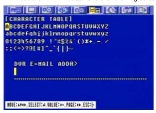
Select the character using the lacktriangle, lacktriangle, lacktriangle, buttons and then press the ENTER button. To exit this CHARACTER TABLE screen, press the ESC button
