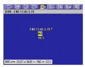
If you want to initialize, move the cursor to "YES" and then press the ENTER button. If not, move the cursor to "NO" and then press the ENTER button. Use the ♠ , ♣ buttons to move the cursor. To exit this DVR INITIALIZE screen, press the ESC button.
