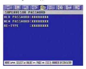
Insert the current password in the eight digits marked \*\*\*\*\*\*\* beside OLD PASSWORD using the CAMERA/ NUMBER INPUT buttons.
