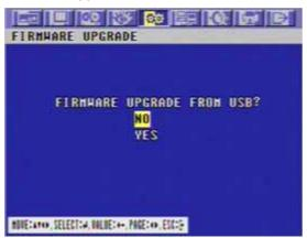
If you want to update firmware using the USB\_FRONT port, move the cursor to "YES" and then press the ENTER button. If not, move the cursor to "NO" and then press the ENTER button. Use the ♠ , ♣ buttons to move the cursor.
