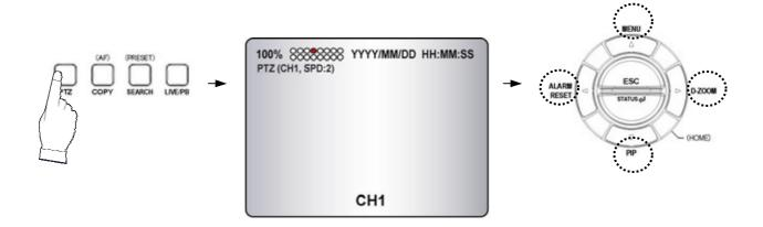
Press the "PTZ" button to control pan, tilt and zoom functions of PTZ camera.
